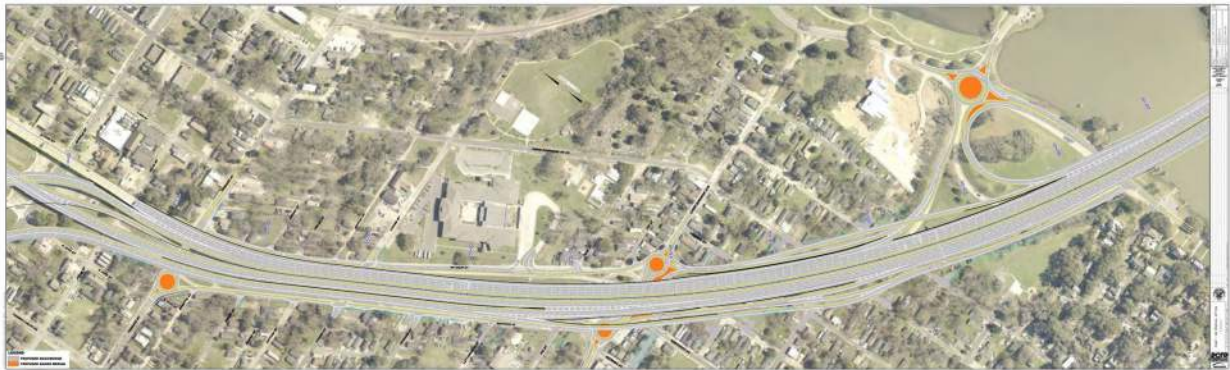
Figure 13. Adopted Refinement: I-10 WB Entrance Ramp from Lorri Burgess Avenue is Removed
