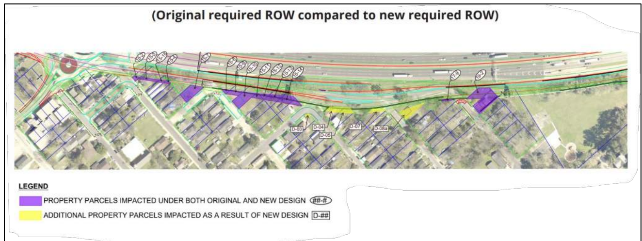
Figure 9. Overview Map of Additional Right of Way Required for I-10 EB Refinement
