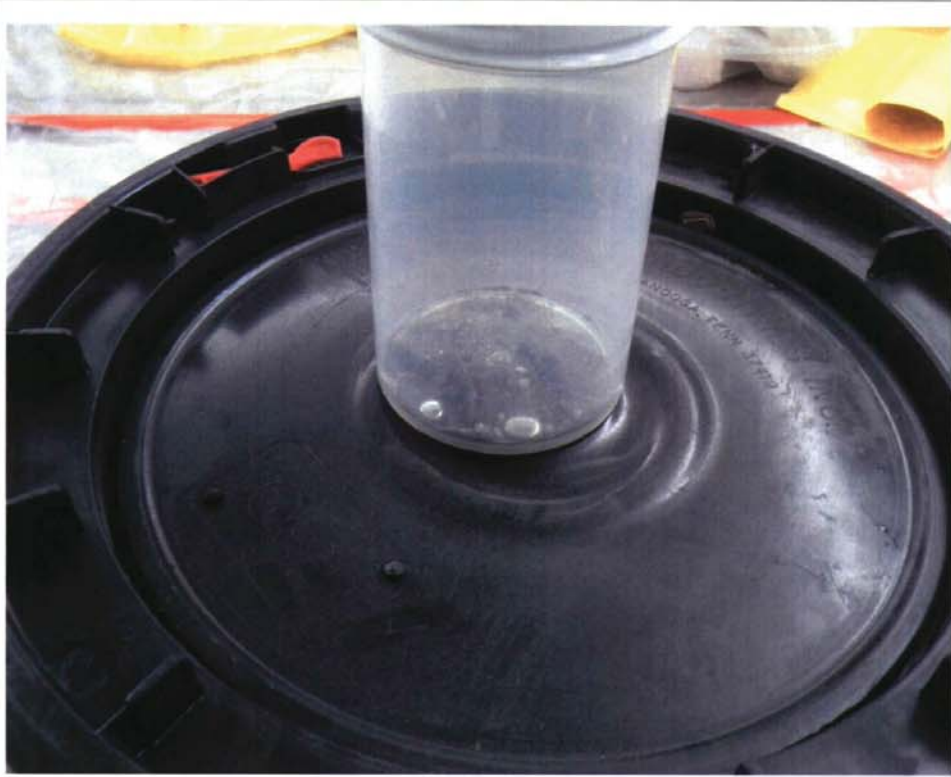
Photo #: 3 of 3 Time: 8/10/2011 Description: view of elemental mercury collected by ERRS with mercury vacuum
